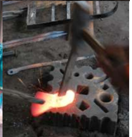
Forging a side axe from a lorry half-shaft - ITAHWA BLACKSMITHS
