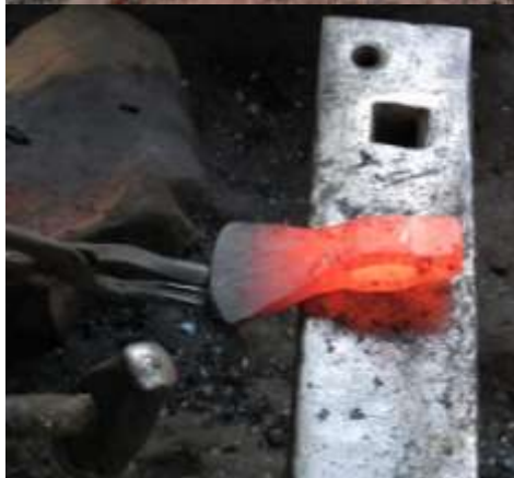
Forging a side axe from a lorry half-shaft - ITAHWA BLACKSMITHS
